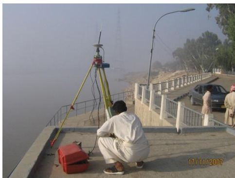
GPS Master Station set up one of the abutments
