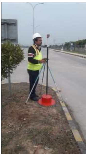
Surveyor with prism at survey benchmark on landside
