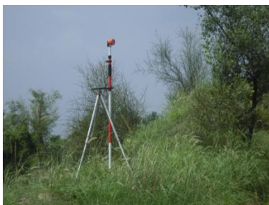
Reflector Prism on Station
