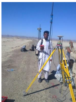
GPS Base Station
