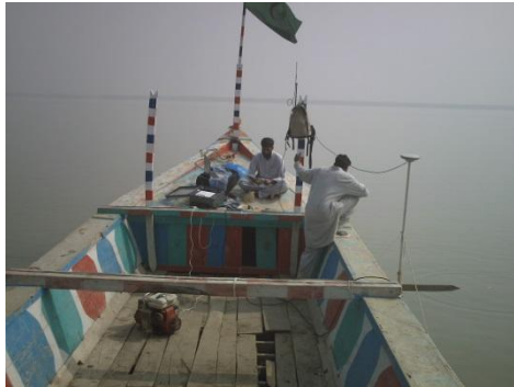
Local boat fitted with Echo Sounder and GPS
