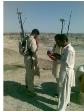
Topographical data acquired via RTK mode
