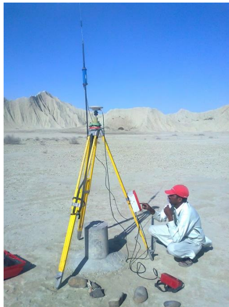
GPS Base Station
