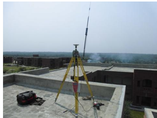
GPS Base Station
